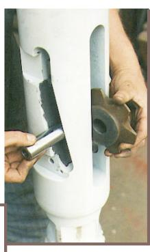
**Adapters** slide onto the back of the perforator body and bolt to the holes which line up on the sides of the perforator.
