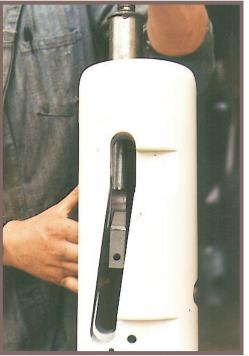
Step 7. Place cutter wheel into perforator body and slide axle pin through cutter wheel.
