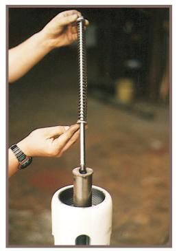
Step 4. Slide chrome rod through spring with a washer on each side of the spring. Install the rod through the cylinder and piston.
