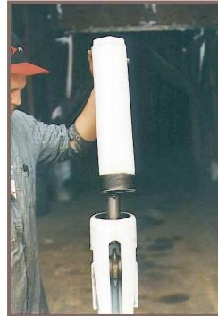
**Step 12.** The pop off valve is installed as one unit by threading it into the lower housing.
