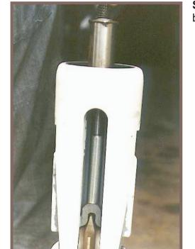
Step 8. Slide cutter wheel and axle pin up into yoke. Insert axle pin bolt through yoke and tighten.
