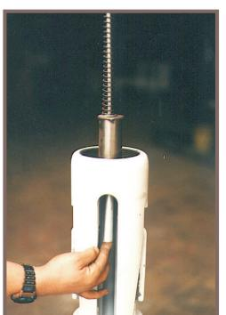
**Step 5.** Place the stop tube between the piston and the yoke.
